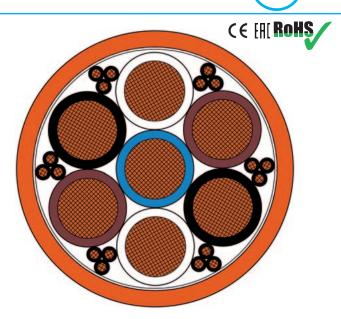
Application: For use as fixed installation cable in 400 Hz systems, e.g. between 400 Hz generator and cable dispenser.
